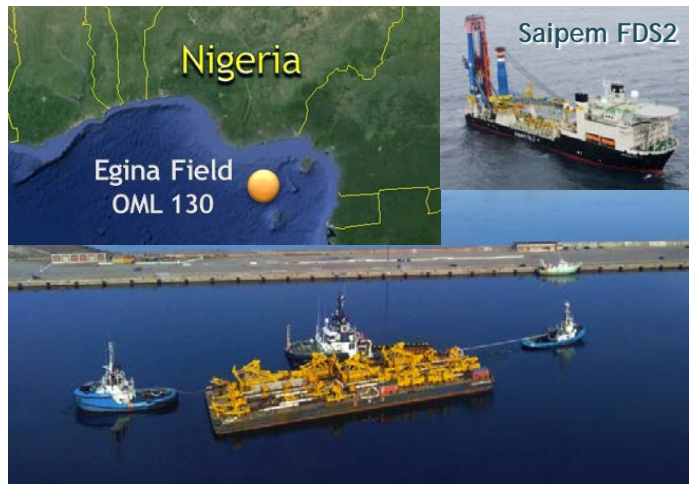
Departure from yard of the top/bottom part of the riser
